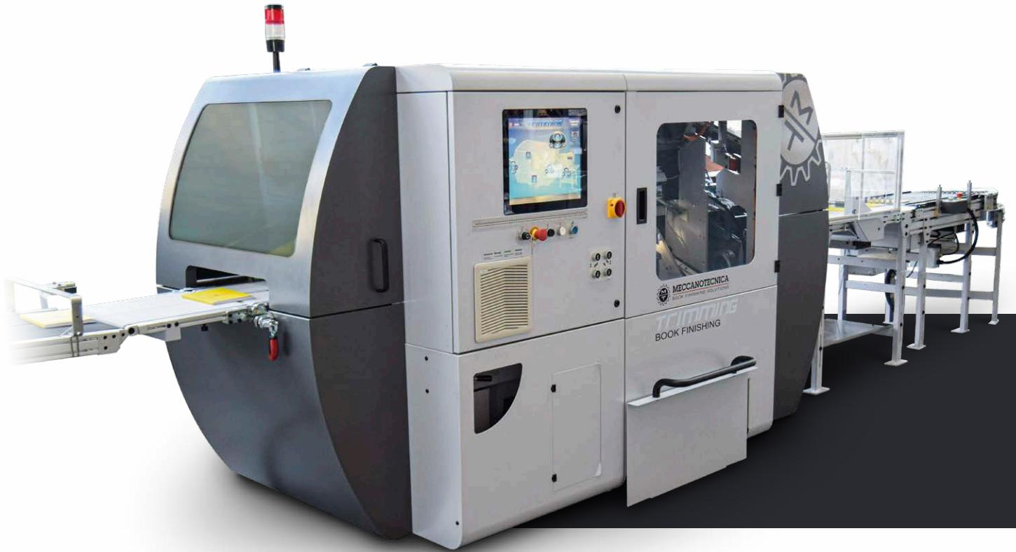
**Trimming**, the automatic three-knife trimmer performs fully variable changeovers producing books in short runs, down to one copy, even with flaps.
